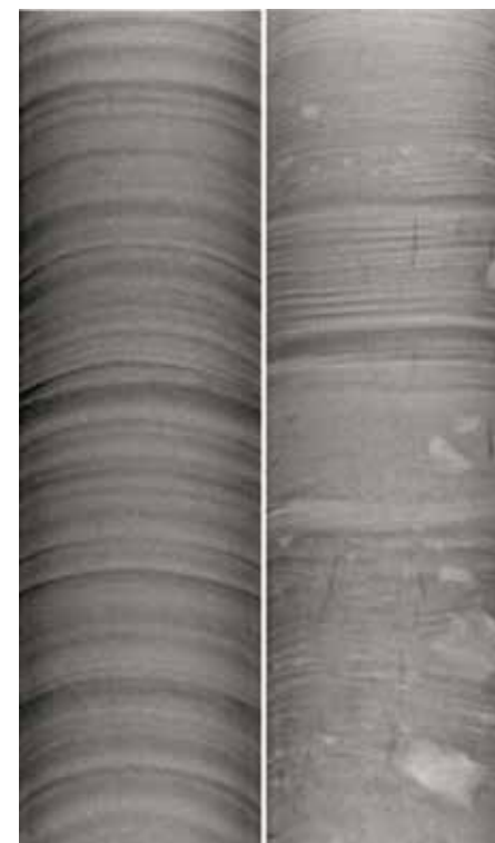
X-ray images of sediment cores showing 30 mm of annual layers and drop stones (left: near the surface, right: just above the ice age gravels)
