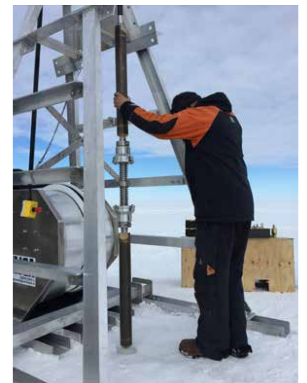
Melting a hole through the ice during the Hot Water Drill commissioning field season, Windless Bight, Antarctica Photo: Jiwoong Chung (KOPRI)
