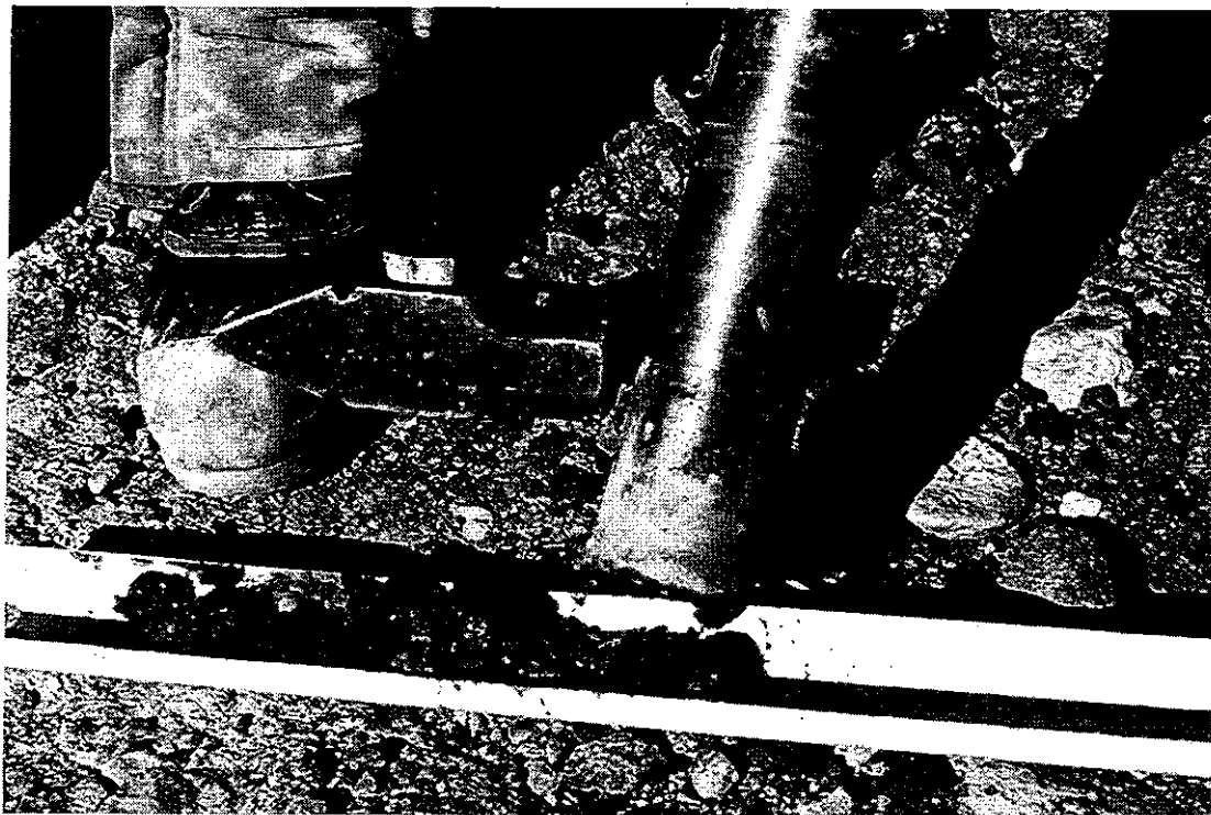
Figure 3 Extracting muddy core from the ice-cemented zone by hammering on the core barrel before the paste can freeze.
