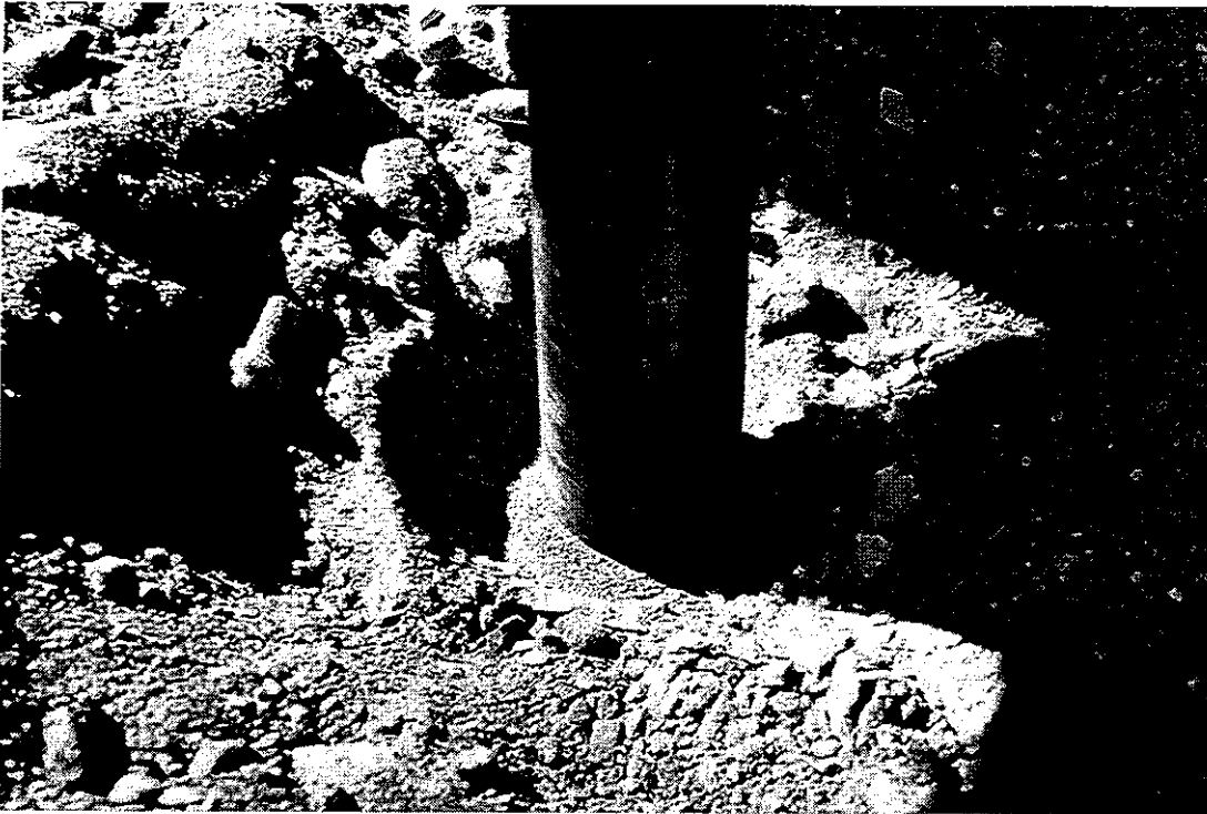
Figure 2 Drilling into the uncemented surface horizon without compressed air at Mt Feather shows the core being pulverized.
