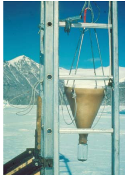
Figure 9. Sediment trap built by Alex Pyne with assistance from Rob Dunbar, Rice University.
