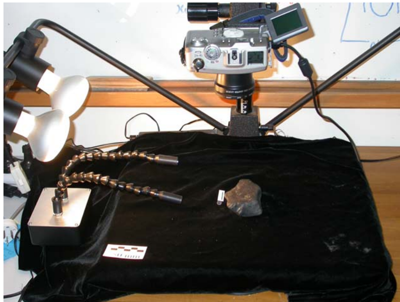
Figure 3 Camera and lighting stand used to generate digital images of clasts. The camera is mounted vertically and the clast is illuminated from one side.
