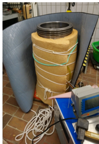
Insulating the cooled salt water tank
