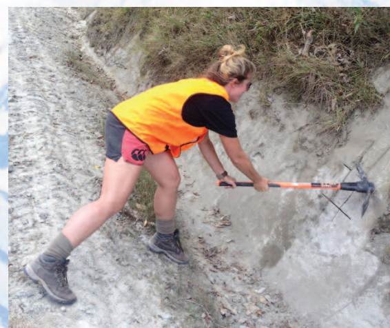
Juliet Sefton aligning a hack into a carefully-cut mudstone block
