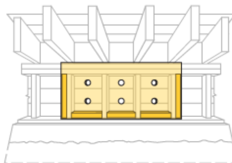
Typical Cripple Wall Bracing Plywood Panel with air vent holes, Double Studding and Blocking
