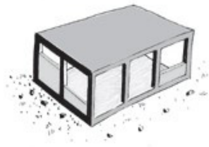
RC frames with infill walls: concrete frame first, walls later
