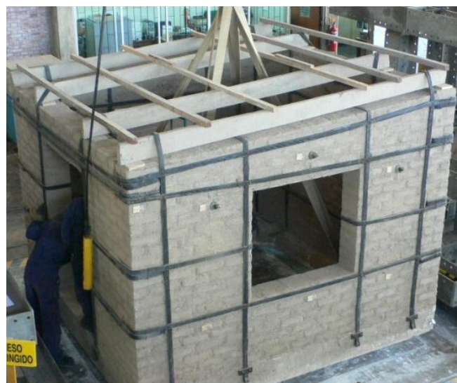
Fig. 11 The adobe test module on the shaking table.
